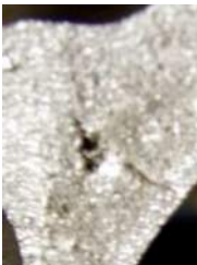
Illus. 4: Shrinkage cavity
