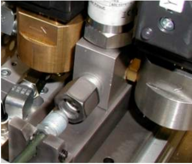
Illus. 27: Sealing from the front with support of the specimen with help of the fixture
