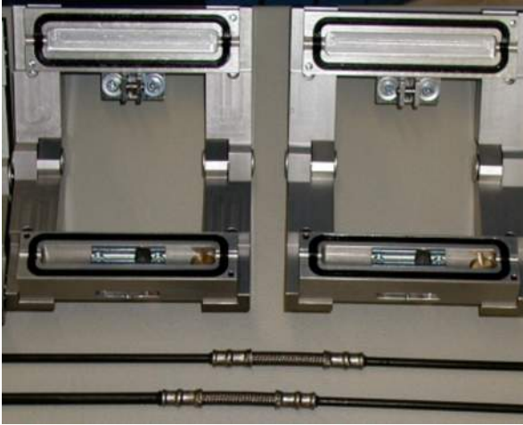
Illus.14: Test hoods for pressure build-up method
